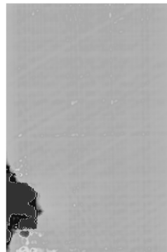
Sample: 12-layer Laminate with delamination (90°/0°/120°/30°/150°/60°/60°/150°/30°/120°/0°/90°) b*h*t: 10*18*0.5cm
